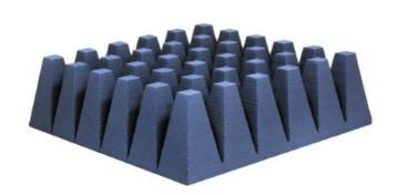
ETS-Lindgren's FerroSorb FS-200 is part of the FS Family of hybrid (ferrite tile and carbon loaded material) absorbers. The FAA-200 loaded foam part is designed to match the impedance of ETS-Lindgren's FT-1500 Ferrite Tile Panel. When combined, these two absorber technologies become the FS-200 absorber system.
